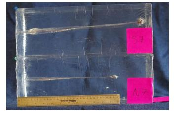
FIG. 3—A representative pair to demonstrate bullet penetration into ballistics gel without (S7) and with (N7) an implant.
