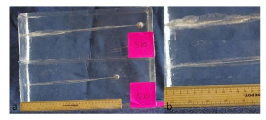
FIG. 4—(a) Representative pair to demonstrate timing of mushrooming without (S10) and with (N10) an implant. (b) Close up of entrance to gel, demonstrating mushrooming within the gel in nonimplant group (S10, upper) and mushrooming prior to gel entry in implant group (N10, lower).
